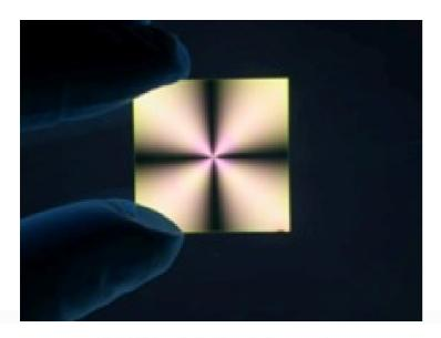
PIAACMC optimized focal plane mask F/20 beam, 10% bandwidth around 0.5 μm SiO2, 20 zones, 4 μm max deviation
