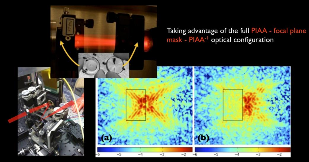
SCExAO's PIAA coronagraph permits speckle control from 1.5 to 14  $\lambda$ /D Raw contrast ~ 3e-4 inside the DM control region Martinache et al, 2012, PASP, 124, 1288
