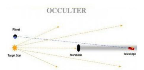
A properly placed and shaped occulter can drop a deep shadow of starlight over a telescope while allowing planet light to pass unimpeded.
