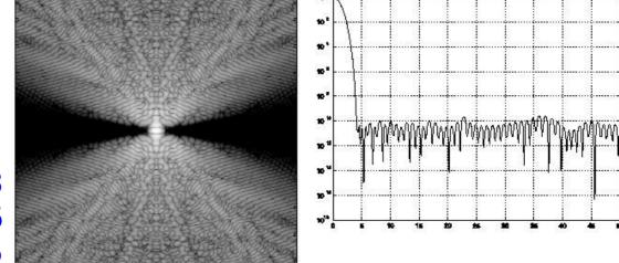
FiG. 9.—*Top*: Asymmetric multiopening mask designed to provide high-contrast,  $10^{-10}$ , from  $\lambda/D = 4$  to  $\lambda/D = 100$  in two angular sectors centered on the x-axis. Ten integrations are required to cover all angles. Total throughput and pseudoarea are 24.4%. Airy throughput is 11.85%. *Bottom*: Associated PSF. (Note that this mask was originally designed for an elliptical mirror. It has been rescaled to fit a circular aperture.)
