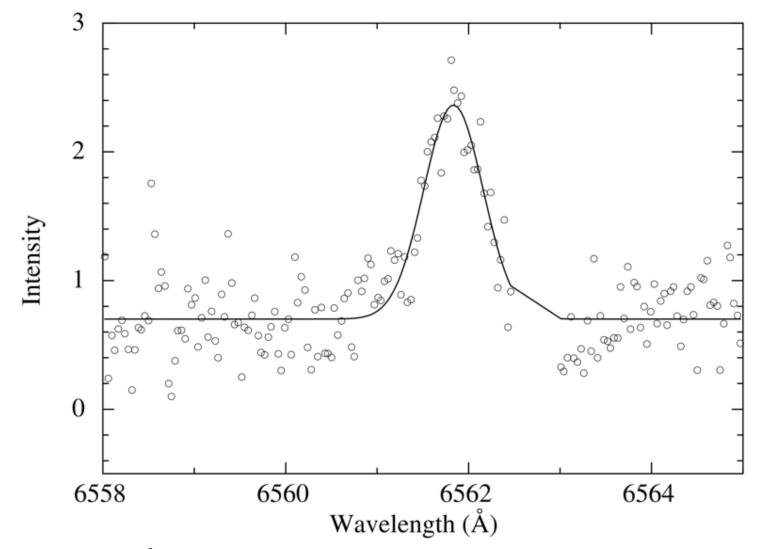
□ Line center:  $6561.8\text{\AA} \rightarrow$  Heliocentric l.o.s velocity of -33 km/s
