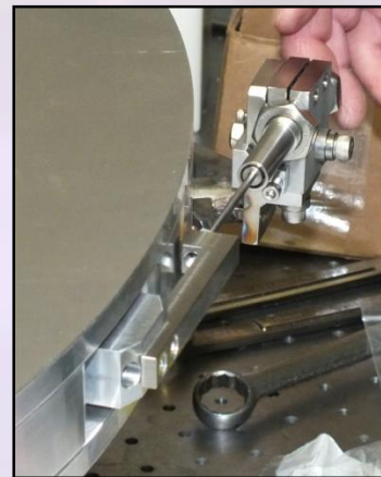
Mirror Support Flexure
