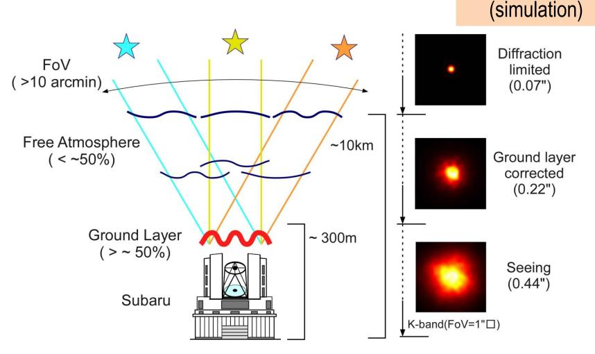
Multiple guide stars are required to determine the ground layer strength
