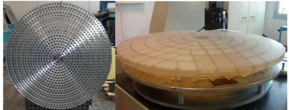
Figure 6: Left: the cold-plate. Right the Zerodur reference body: this optical component is manufactured by SESO (France) and an intricate light-weighting scheme brings the weight of this component to a mere 47 kg.
