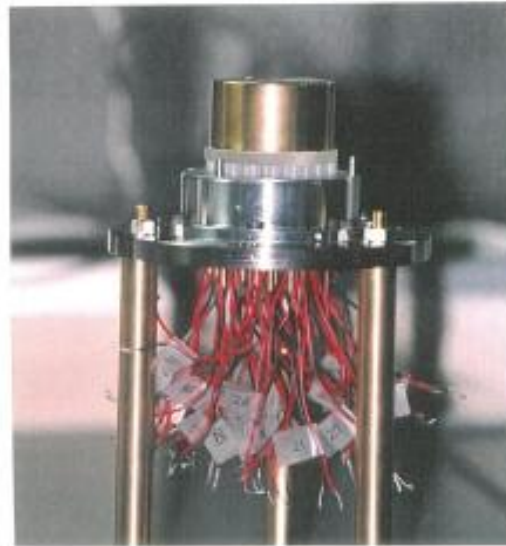
Figure 4.20: Cementing the actuator heads.
